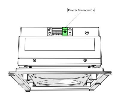
Note: The SCRS-5iw is shipped from the factory wired for passive operation. These instructions are for hookup in that mode. If you intend to run your SCRS-5iw in bi-amp mode, please call the factory for assistance as it will be necessary to change the internal wiring of the speaker.
