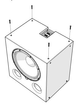
1b. Place HF Unit on LF Unit, aligning front-to-back, side-to-side
