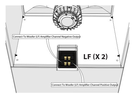
Note: The two pairs of binding posts on the LF units are wired together inside the loudspeaker, therefore, either set may be used, or you may use all four to increase current capability by using four wires from your amplifer. If you use four, connect the two negative wires together and the two positive wires together at the amplifier end and then to the corresponding amplifier output terminal.
