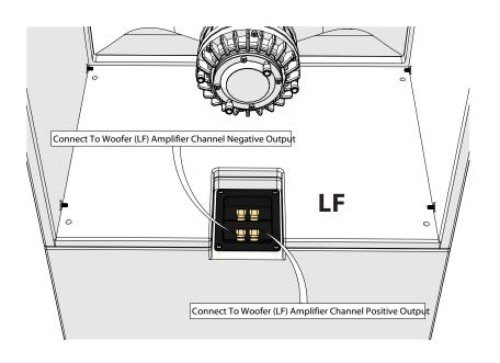
Note: The two pairs of binding posts on the LF unit are wired together inside the loudspeaker, therefore, either set may be used, or you may use all four to increase current capability by using four wires from your amplifer. If you use four, connect the two negative wires together and the two positive wires together at the amplifier end and then to the corresponding amplifier output terminal.
